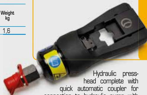
Hydraulic press-head complete with quick automatic coupler for connection to hydraulic pump with working pressure of 700 bar max, (see page 170-174). RHM50 is suitable for installing the same range of connectors as RH50.
