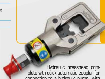
Hydraulic presshead complete with quick automatic coupler for connection to a hydraulic pump with a working pressure of 700 bar max, (see page 170-174) RH 50 is suitable for installing the same range of connectors as HT 51.
