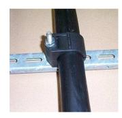
4) Important: Do not over tighten the clamp. The clamp should secure the cable but does not need to be so tight that the cable bulges at either side of the clamp or becomes angled excessively.
