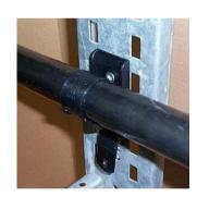
4) Pass the end of the retaining strap through the two legs below the cable support to lock the strap. To release the strap use a screw driver to prise open the legs.
