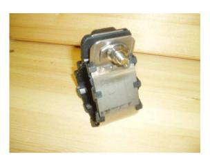
Replace the Flange nut. Tighten until sufficient tension is achieved.
