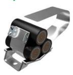
Fasten base to support with M10 fixings. Loop strap through base and around cables. Standard duty = 2 loops. Heavy Duty = 3 loops.
