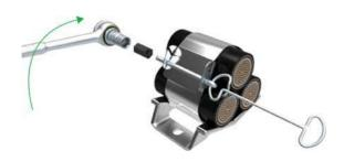
Pull slack into outer loop. Insert split pin from right hand side around outer layer of strap about 10mm from end. Push plastic shear torque adaptor fully onto the end of the split pin and attach 13mm socket wrench. To tension the strap rotate key anti-clockwise with the socket wrench until the adaptor shears.
