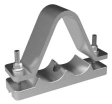
The orion cleat provides the strongest support for cables laid in trefoil formation. Suitable for LV, MV and HV cable designs, the orion cleat features deep cast bases to aid easy cable installations.
