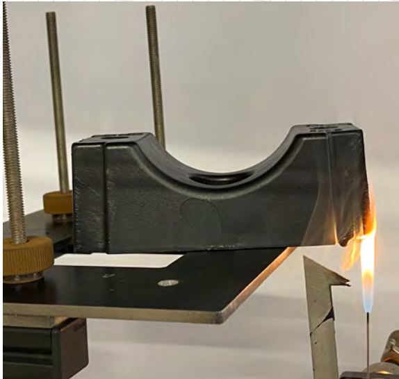
FLAME PROPAGATION TEST ON SOLUS NON-METALLIC CLEAT.
