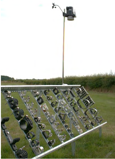
IN ADDITION TO THE CORROSION TESTING TO IEC 61914 ELLIS CARRIES OUT EXTENDED TESTING ON ITS OUTDOOR WEATHERING STATION.
