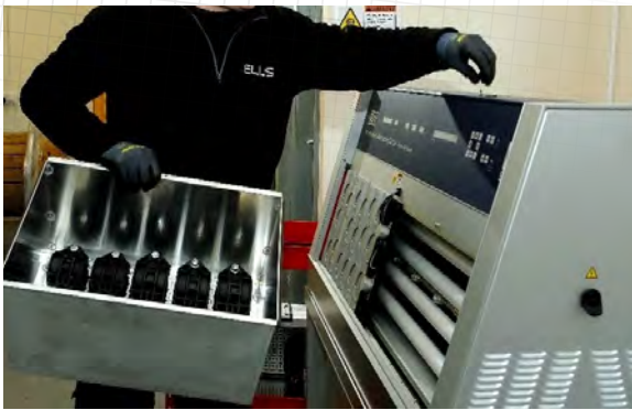
ELLIS' IN HOUSE UV WEATHERING TEST STATION
