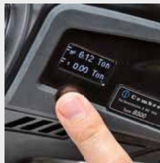
Multifunction OLED display with touch button
