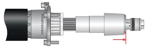
Slide the bell flange onto the insulating part.
