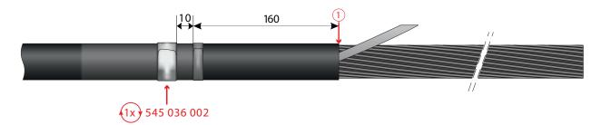
Fold back the screen wires and fix them with insulating tape.
