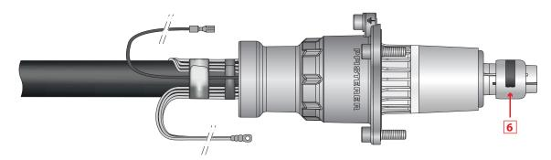
Place the pressure plate [6] on the thrust piece of the compression head and slide the retaining ring of the compression head to the back.
