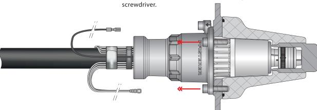
Pull the CONNEX separable connector out of the socket.
