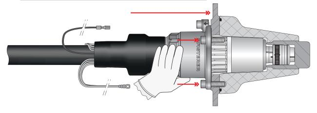
Tighten the screws all round with the SW6 T-handle screwdriver (torque 15 Nm).
