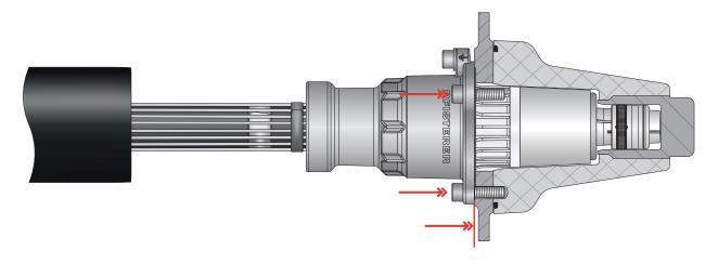
Using the ruler, check the position of the contact to confirm the dimension 207 mm; otherwise press the cable again.
