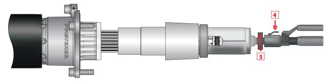
17 Press the contact ring onto the tension cone with the hydraulic hand-operated compression tool until it reaches pressure.
