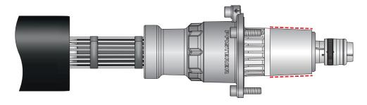
Introduce the CONNEX separable connector into socket and tighten the screws.
