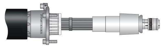
Fix the contact ring onto the tension cone with the impact device.
