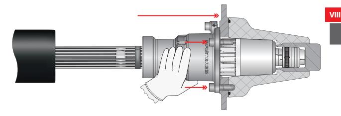
Tighten the screws going around on alternating sides to a torque of 15 Nm.
