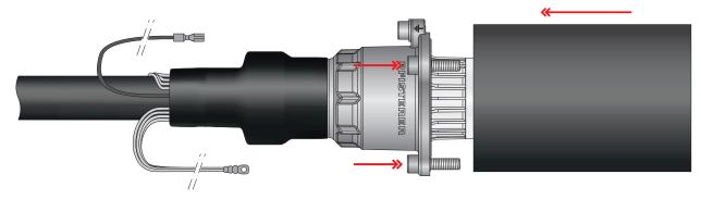
Clean the inside of the socket and wait until the cleaning agent has fully evaporated. The recommended cleaning agent is white gasoline or acetone, see chapter 3.9, page 10.
