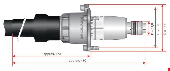
Size 3 | 3-S Length, including heat-shrink tube [mm] approx. 460 Outer diameter, max. 148 [mm] Hole circle [mm] 130 Weight / part [kg] approx. 3.3 54.8 Contact ring [mm]
