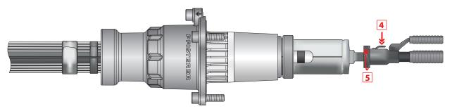
Pull the contact ring off the tension cone with the hydraulic hand-operated compression tool.
