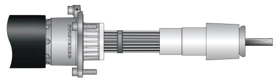
11 Slide the tension cone onto the conductor up to the thrust piece.
