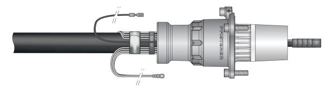
Remove the insulating part and bell flange.
