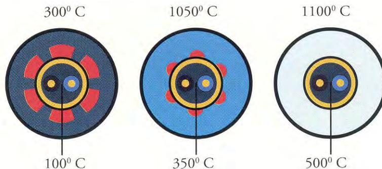
When this process is completed, the layer will turn into a firm, ceramic substance which provides heat insulation. Consequently, this is why the conductor temperature can be kept at a low level (approx. 500°C/900°F) even if the temperature should exceed 1100°C (2000°F). For Instrument and Communications applications, the values of Capacitance, Inductance, Resistance and Attenuation are not unduly affected.
