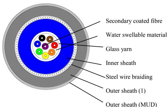
An additional outer sheath is added for improved oil- and MUD protection. The outer sheath is DARK GREY.
