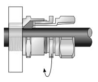
6. Attach the conduit to the Conduit Coupler (5) and fully tighten. Ensure that the Seal Nut (4) does not come loose during this process by holding it with a spanner.
