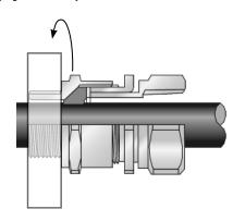
4. Determine the conductor length required to suit the installation and prepare the cable accordingly, removing part of the outer sheath where required to reveal the insulated conductors.
