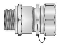
3. Fit the gland into the equipment and fully tighten the Entry Item (1).
