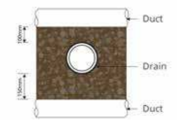
Minimum clearance between duct and drain
