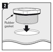
Insert the sleeve. Make sure the rubber gasket is in place.
