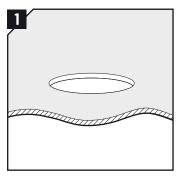
Make a hole for the sleeve, according to the rec. hole cut. See table on next page.
