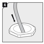
Insert the cable/pipe through the sleeve.
