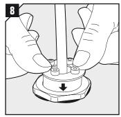
Place the seal around the cable and insert it into the sleeve.
