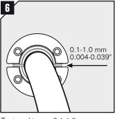
Try to achieve a 0.1-1.0 mm gap between the two halves when held against the cable/pipe.
