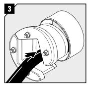
Insert the frame into the sleeve opening.
