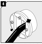
Loosen the nuts and push the front fittings to the sides.
