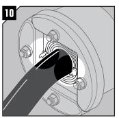
Excess Roxtec Lubricant will protrude when tightening the seal.
