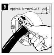
Tighten the nuts. Max torque is 4 Nm/2.95 lbf-ft.
