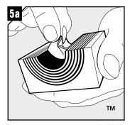
Adapt modules which are to hold cables or pipes by peeling off layers until you reach the gap seen in pic. 5b.
