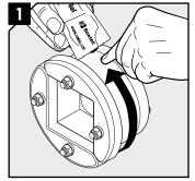
Lubricate the frame sparsely on the outside black rubber part with Roxtec Assembly Gel.
