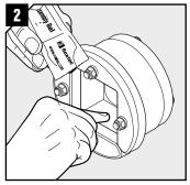
Lubricate the inside faces of the frame thoroughly, especially into the corners.
