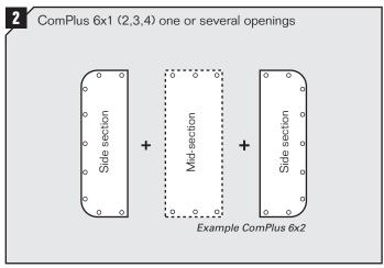
To assemble, remove all protective tape from gaskets and fit two frame sections together. To add openings, just add frame mid-sections.
