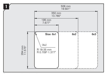
Cut a hole in the cabinet/wall according to the picture above.
