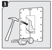
Knock-out the protective cover from the front to prepare the frame for installation.
