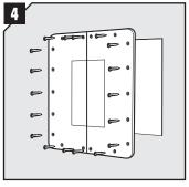
Attach to wall using (self-tapping) screws or rivets. Recommended screw dim. ST 5.5.
