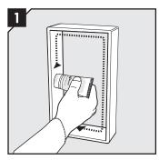
Lubricate the inside surfaces of the frame with Roxtec Assembly Gel, especially into the corners.
