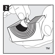
Adapt modules, which are to hold cables or pipes, by peeling off layers until you reach the gap seen in pic. 3. The halves may not differ by more than one layer.
