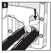
Insert the modules according to your installation plan (transit plan). It is recommended to seal cables/pipes at the bottom of the frame and put spare modules on top.
