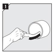
Remove any dirt in the sleeve/hole.
