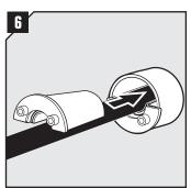
Insert the halves into the sleeve.
