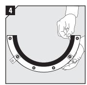
Adapt the seal to the cable/pipe by peeling off layers from the halves until you reach the gap seen in pic.5. The halves may not differ by more than one layer.
