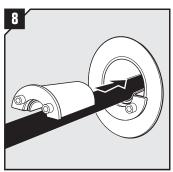
Insert the halves into the sleeve.
