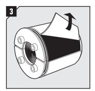
Adapt the seal to the sleeve/ hole by peeling off layers from the halves until you reach the right outer diameter.
