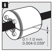
Try to achieve a 0.1-1.0 mm gap between the two halves when held against the cable/pipe.
