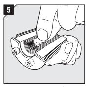
Adapt the seal to the cable/pipe by peeling off layers from the halves until you reach the gap seen in pic.6. The halves may not differ by more than one layer.
