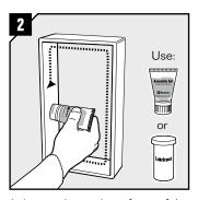
Lubricate the inside surfaces of the frame with Roxtec Assembly Gel or Roxtec Lubrucant, especially into the corners.
