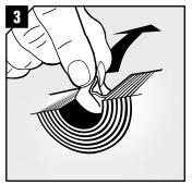
Adapt modules which are to hold cables or pipes by peeling layers until you reach the gap seen in pic. 4.
