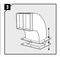
Attach the frame to the roof using bolts/bolts and nuts. The rubber gasket shall be placed between frame and roof.
