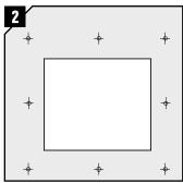
Use the frame as template for the drilling of the screw holes. Hole in frame  $\emptyset = 12 \text{ mm } (0.472)^\circ$ .
