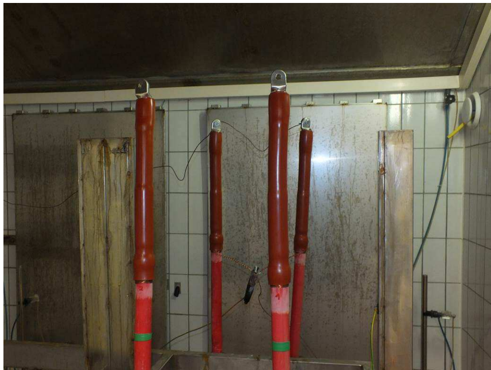
Figure 3: Test set up of the humidity test
