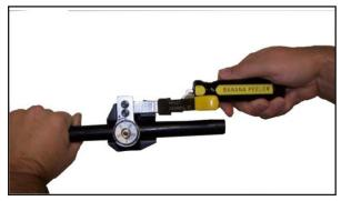
2. Turn tool 90 degrees, depress lever, and position blade so it seats in the scored groove you created with the first operation. Release lever and draw the tool lengthwise off the end of the cable. Repeat this procedure several times around the cable, as required. Some sheathings are more tightly bonded to the insulation than others and more longitudinal scores makes their removal easier.
