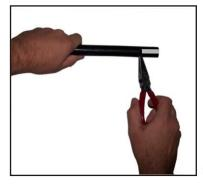
3. Peel scored semi-con segments with needle nose pliers or other suitable tool. Perfectly scored semi-con is cleanly removed without damage to underlying insulation.
