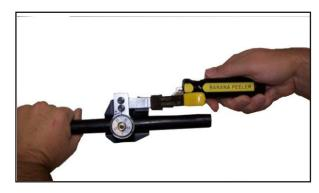
2. Turn tool 90 degrees, depress lever, and position blade so it seats in the scored groove you created with the first operation. Release lever and draw the tool lengthwise off the end of the cable. Repeat this procedure several times around the cable, as required. Some sheathings are more tightly bonded to the insulation than others and more longitudinal scores makes their removal easier.
