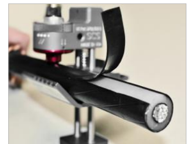
Simply pull the tool along the full cable length to perform longitudinal cuts.
