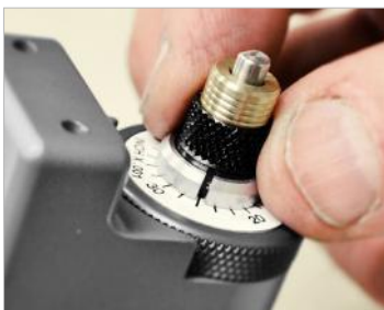
Blade depth is easily adjustable & set by turning the dial.
