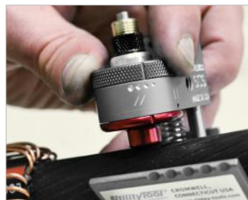
Four blade pitch settings adjust the spiral width for various cable sizes.
