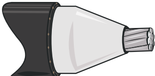
PENCILING INSULATION ON URD CABLE
