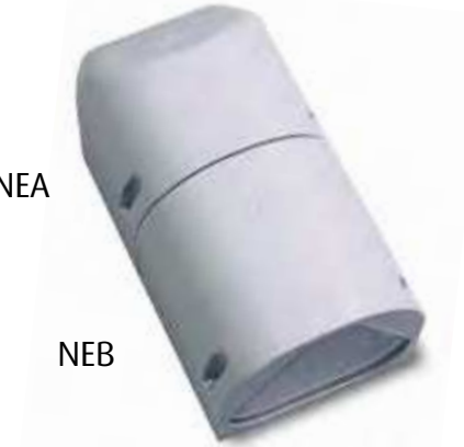
Extension Trough NEC, 3 entry Created by coupling NEA trough to NEB Terminals can be installed in either upper chamber (NEA) or lower chamber (NEB). Length 180mm, Width 98mm, Depth 93mm
