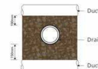
Minimum clearance between duct and drain
