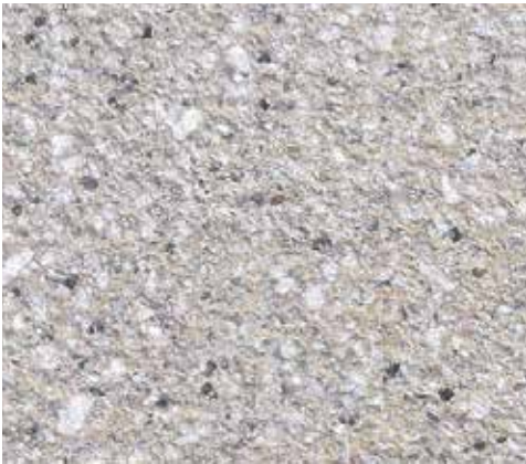
Exposed aggregate finish
