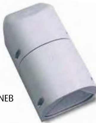
Extension Trough NEC, 3 entry Created by coupling NEA trough to NEB Terminals can be installed in either upper chamber (NEA) or lower chamber (NEB). Length 180mm, Width 98mm, Depth 93mm
