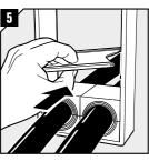
Insert a stayplate on top of every finished row of modules.
