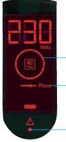
Rotary Field indicator. Unipolar identification of the phase.
