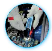
Voltage detection on electrical power circuit.
