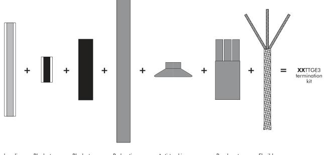
Red sealing mastic "MBA" Black stress control mastic "MACDC" Black stress control tube "GT1" Red antitracking tube "GT2" Anti-tracking sheds
