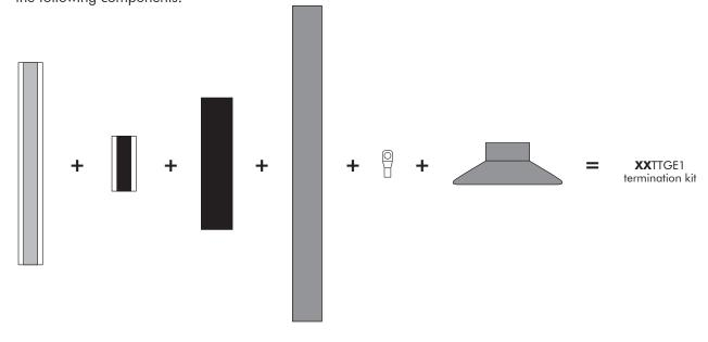
Red sealing mastic "MBA" Black stress control mastic "MACDC" Black stress control tube "GT1" Red antitracking tube "GT2" Earthing lug for screen wires
