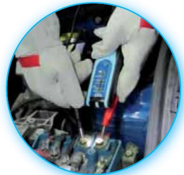
Voltage detection on electrical power circuit.
