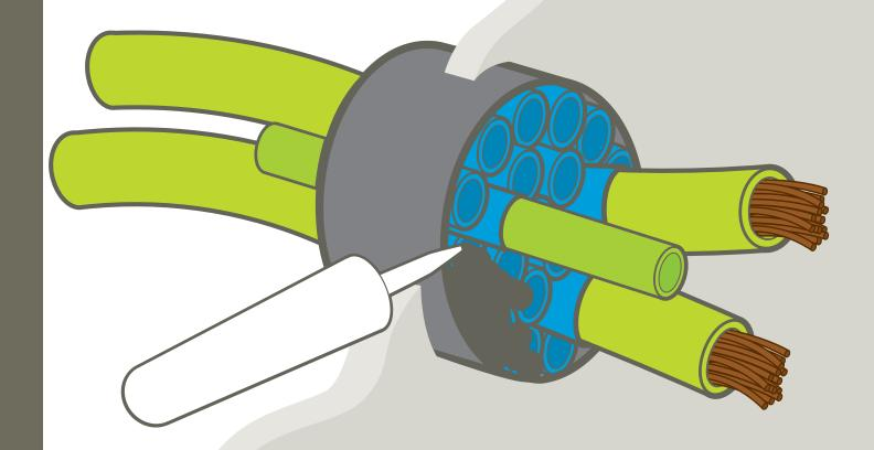
"...an effective and simple solution to gastight and watertight sealing requirements."
