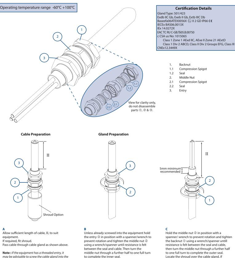
may be advisable to screw the cable gland into the equipment to prevent twisting of the cable after Step B & C.
