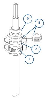
Remove entry ® and refit inner seal \$, replace entry © and re-assemble middle nut ② onto the entry component ©. Tighten up the middle nut ② using a wrench/spanner until resistance is felt between the seal and cable, then turn the middle nut through a further half a full turn to complete the inner seal.
