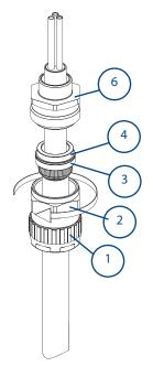
Unscrew the middle nut ② and visually inspect that between the armour spigot @ and the armour clamping ring ③. If armour/braid not clamped, repeat assembly.
