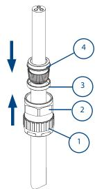
Push the cable through the armour spigot ④. Spread
