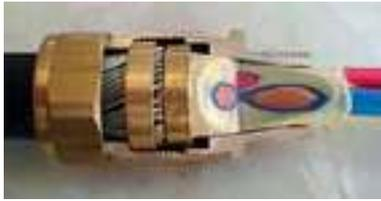
To maintain the integrity of the type of protection thread engagement must be at least five full threads. Suitable grease may be used provided it is nonsetting, non-metallic and non-combustible and any earthing between the two is maintained. Where taper threads are used, the connection shall be made wrench tight.
