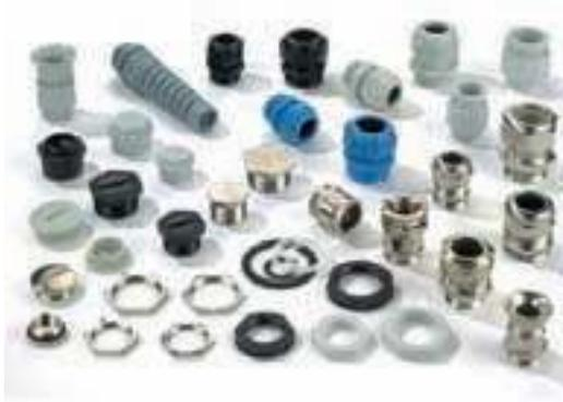
Cable glands must maintain at least IP 54. The cable glands require an EC Type Examination Certificate by a Notified Body for the protection type increased safety Ex e. For example a certification for flameproof Ex d only is not sufficient for increased safety Ex e certified enclosures. Cable glands are typically equipment certified.
