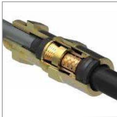
**The Excel plus in a universal hazardous area cable gland achieves IP67 and deluge protection with additional features for soft - bedding materials subject to cold flow.**
