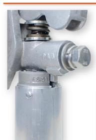
Clamp 'NIB' engages in the S9D socket to locate the clamp whilst being raised into position. The clamp does not require being fully opened/unscrewed as the socket controls the clamp whilst being fitted over the busbar.
