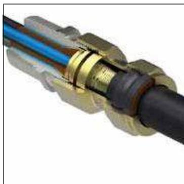
The Barr X is an explosion proof gland suitable for jacketed marine shipboard cables with braid armor which aids the control of migrating gases and is the best choice when the highest level of protection is required.
