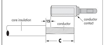
A. Remove the core insulation from the conductor for a distance **« C »** mm (**C** = depth of contact bore + **15** mm).
