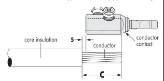
B. Remove the core insulation from the conductor for a distance **« C »** mm (**C** = depth of contact bore + **5** mm).
