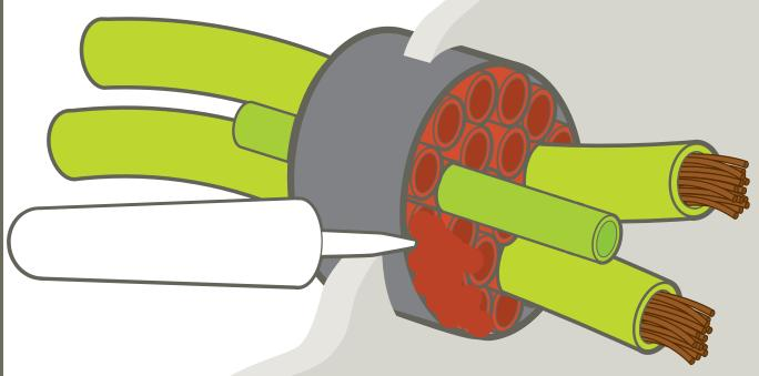
"...an effective and simple solution for sealing cable ducts and building entries against flooding and gas ingress."
