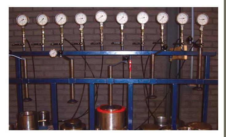
SLIPSIL sealing plugs have undergone through three pressure tests at nominal dimensions to determine the pressure ratings for plugs with smallest, medium and largest of openings.
