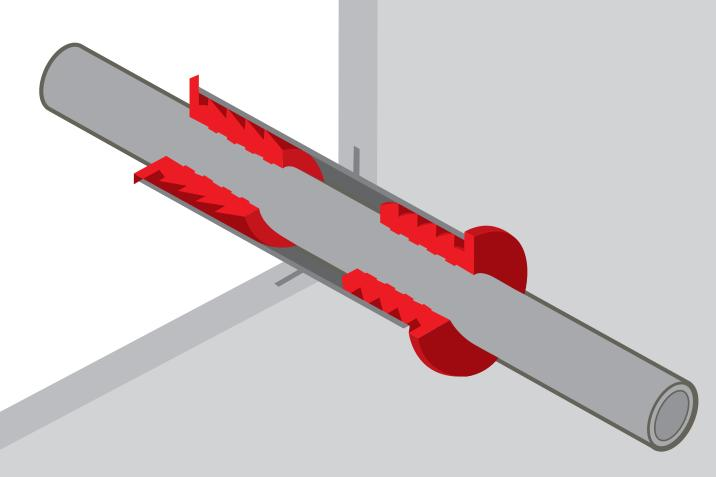
"CSD Sealing Plugs consist of two equal parts that allows them to be inserted after all pipes or cables in a conduit are installed."
