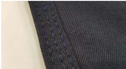
Triple needle stitch seams for extra longevity
