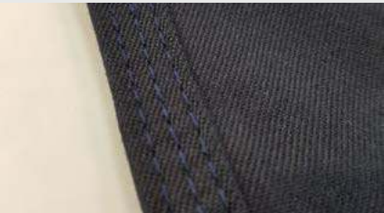
Triple needle stitch seams for extra longevity
