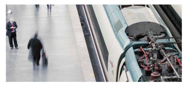
The metal-oxide surge arresters produced by ABB Switzerland Ltd. for DC traction systems are developed and type tested according to the new European standard EN 50526-1 which is specifically for metal-oxide surge arrester in railway application up to 3kV nominal voltage. The surge arresters also meet the requirements for A1/A2 functionality according to VDV 525 recommendation.
