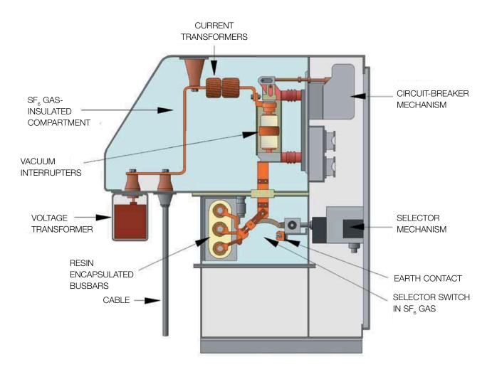
Figure 13 Typical arrangement of a 33 kV fixed-pattern vacuum circuit-breaker with sulphur hexafluoride (SF $_6$ ) gas insulation
