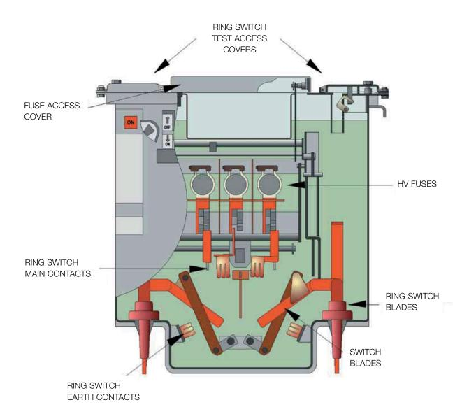
**Figure 11** Typical arrangement of an 11 kV oil-filled common tank ring main unit (incorporating two ring switches and one fuse switch)
