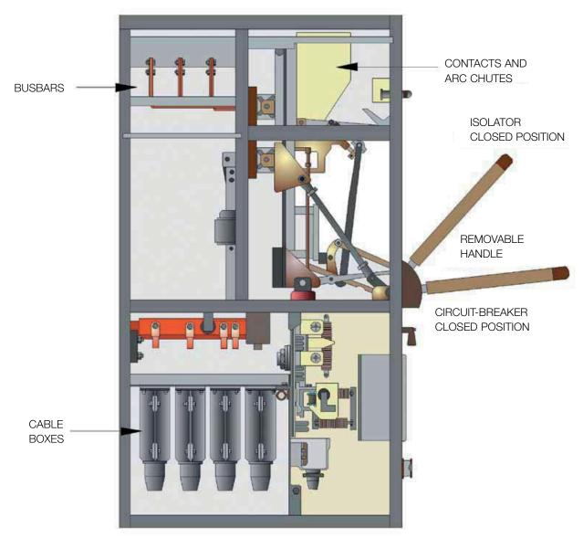
Figure 12 Typical arrangement of a 415 V air circuit-breaker
