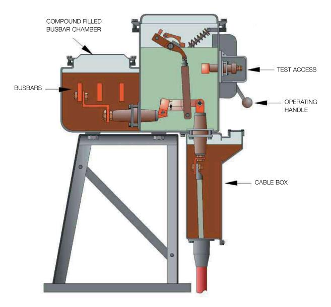
Figure 9 Typical arrangement of an 11 kV oil switch
