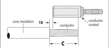
A. Remove the core insulation from the conductor for a distance **« C »** mm (**C** = depth of contact bore + **10** mm).
