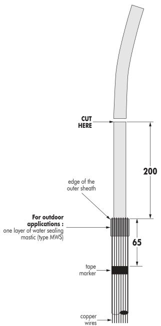
For indoor applications, bend the screen wires back over the outer sheath and proceed to step no. 5.
