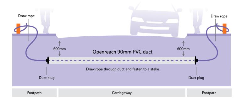
Duct beneath a carriageway crossing must be laid at a depth of 600mm from the cover of the final surface levels. And for engineering reasons (National Joint Utilities Group NJUG) it must be separated from other services laid in parallel by 600mm (to permit us to install underground joint boxes without the need for bends).
