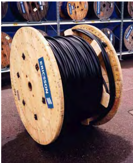
Example of a spare cable on a drum with a long inner end.
