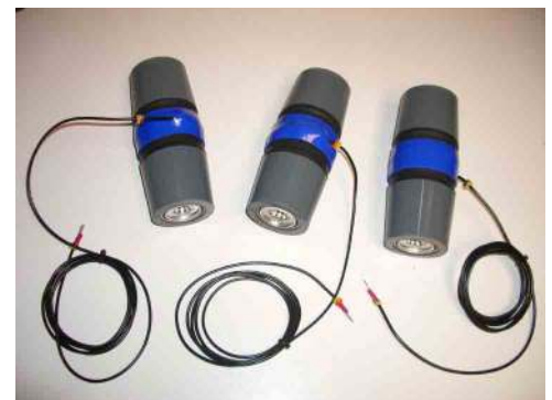
ORMALINK with capacitive output for detection of voltage
